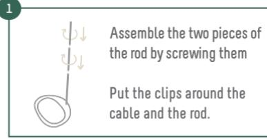
Assemble the two pieces of the rod by screwing them. Put the clips around the cable and the rod.
