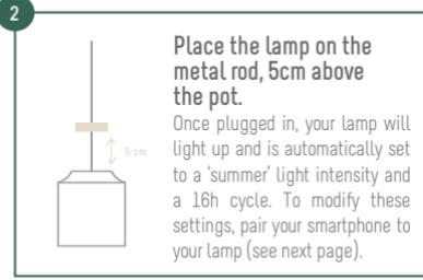
Place the lamp on the metal rod, 5cm above the pot. Once plugged in, your lamp will light up and is automatically set to a 'summer' light intensity and a 16h cycle. To modify these settings, pair your smartphone to your lamp (see next page).
